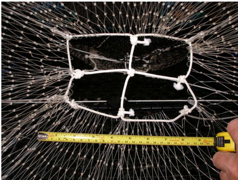
Figure 2.3 Photograph showing the monofilament funnel entrance to the collapsible cod trap, modified with additional twine to reduce the size of the aperture to act as an otter guard.
